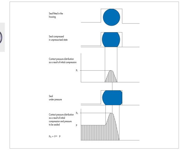
Fig. 9 Automatic sealing effect with elastic seals
