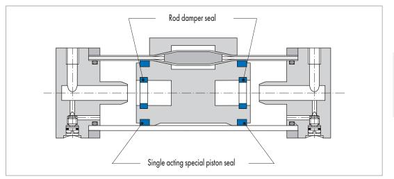
Fig. 5 Pneumatic cylinder without piston rod
