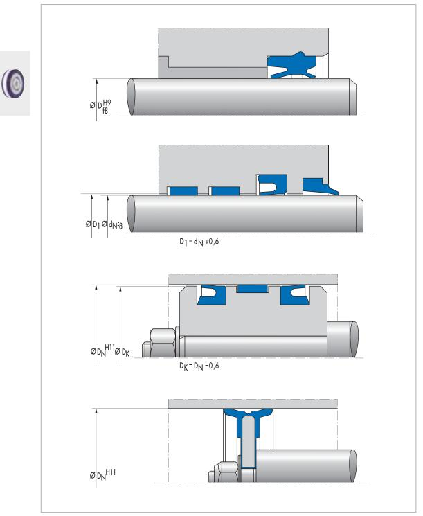
Fig. 16 Fitting and tolerances for seals and guides
