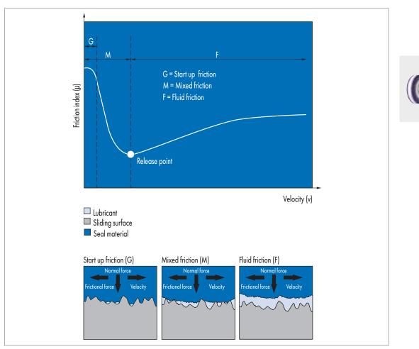
Fig. 12 Stribeck graph describes the dependency of the friction force on the speed
