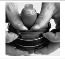
Fig. 26 Snap-in fitting of a piston seal
