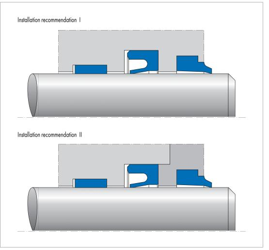
Fig. 20 Fitting types of rod seals
