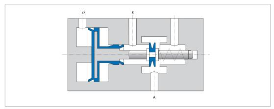
Fig. 7 Pneumatic 3/2-way valve
