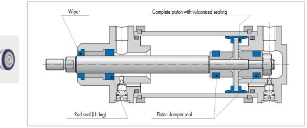
Fig. 3 Pneumatic cylinder II
