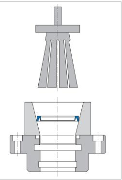
Fig. 23 Fitting of rod seals
