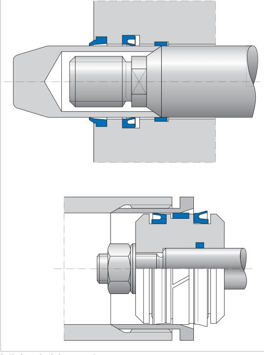
Fig. 19 Covering threads when mounting seals
