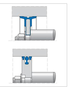
Fig. 28 Assembly of pneumatic complete pistons
