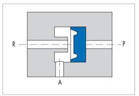
Fig. 6 Pneumatic quick-venting valve
