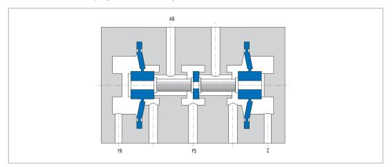
Fig. 8 Pneumatic 5/2-way valve
