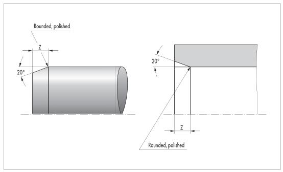
Fig. 18 Chamfering rods and pipes
