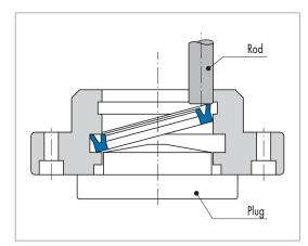
Fig. 24 Fitting aid for rod seals
