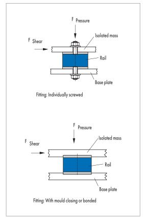
Fitting & installation: rails with load directions
