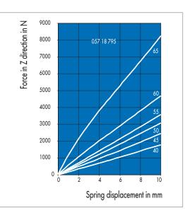
Static spring characteristic curves in Z direction
