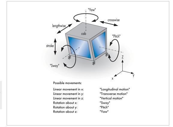
Fig. 1 Possible movements of a rigid body
