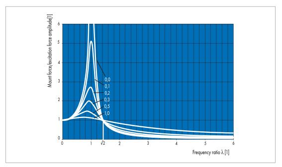
Diagram 2 Amount of the transfer function (quotient resulting from the force reaction and exciter force amplitude)
