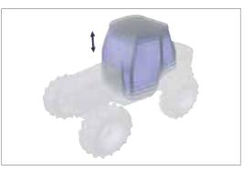
Fig. 5 Vertical vibrations of the cabin before optimisation
