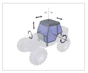
Fig. 4 Movement possibilities of the cabin
