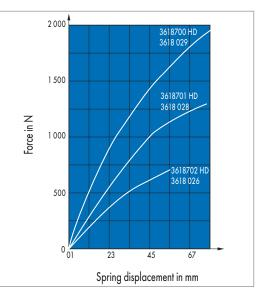
Static spring characteristic curve in Z direction
