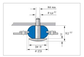
Installation diagram with stud SW19
