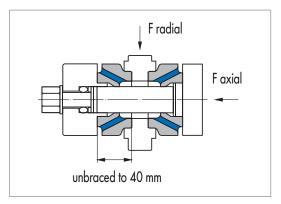
Fitting & installation instructions: Top Mount with load directions
