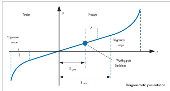
Fig. 8 Working point and oscillation amplitude
