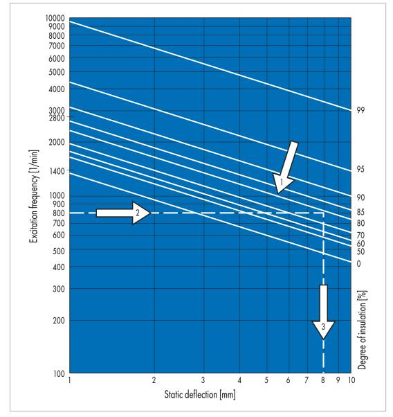
Diagram 3 Determining the static compressive deflection depending on the excitation frequency and the desired degree of insulation
