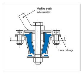
Secured by threaded fasteners in flange
