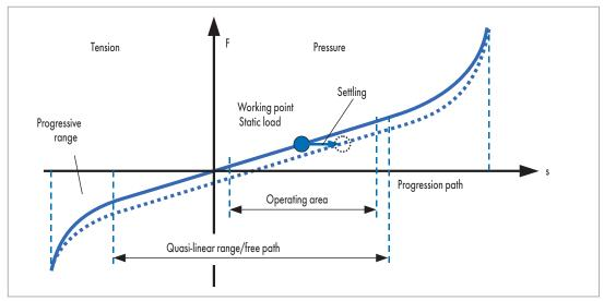
Fig. 9 Settling of elastomeric components
