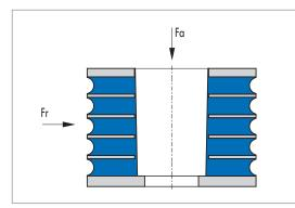
Layered springs have the same stiffness in the radial directions (X and Y direction) and are especially stiff in the vertical direction (Z direction). The effective stiffnesses can be varied by turning of the mount to the static load. Layered springs are designed for the primary load in the axial and radial direction but can also be loaded angled to the vertical primary load. The weight should be absorbed in the longitudinal axis for this.
